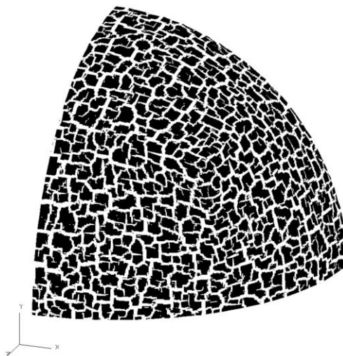
Fig. 10. Demonstration calculation illustrating the type of fracture pattern which can be predicted. 600 000 element mesh of hexahedral elements with five elements through the thickness.
